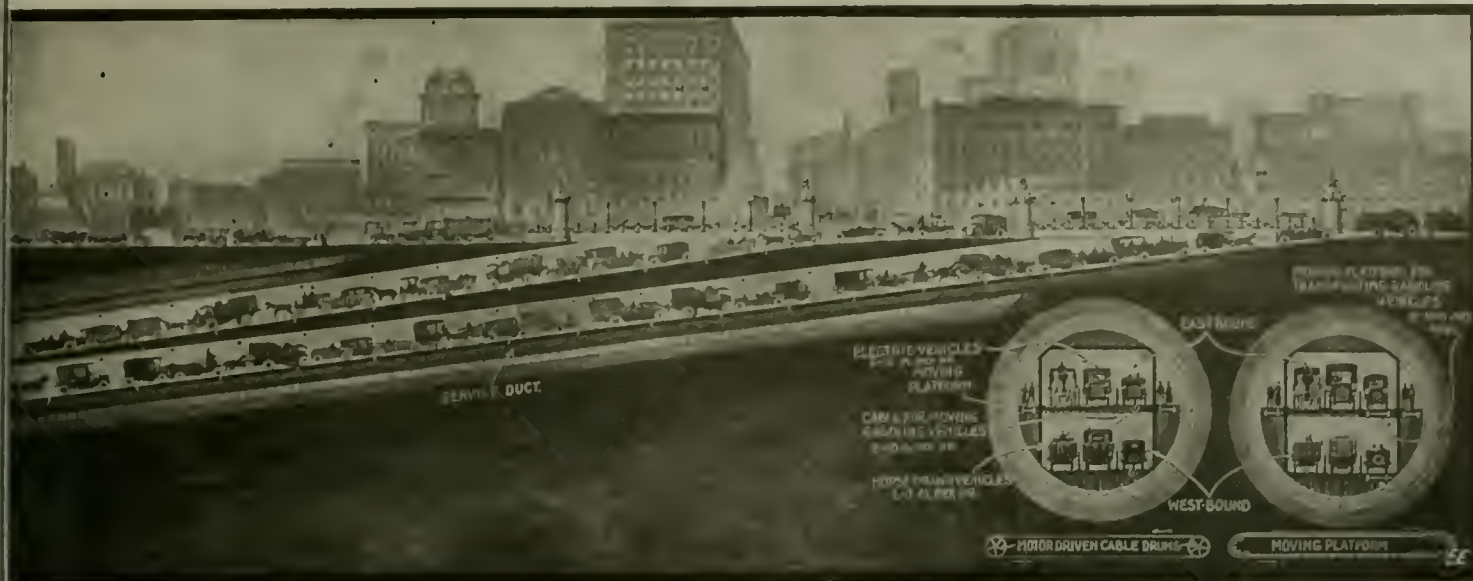
of the Tunnel Project. Among These Features Are the Following:—First, That a Ventilator Shaft be Placed a Comparatively Short Ways Out in the River at Elther Approach, So as to Simplify the Ventilating Problem by Reducing the Length Between the Bulkheads. Second, That Gasoline Vehicles be "Hauled" Thru the Tunnels So as to Eliminate the Fouling of the Air by Obnoxious Exhaust Gases, Particularly Carbon Monoxid, by Means of a Moving Platform. Third, Haul Gasoline Vehicles Thru the Tunnel by a Cableway Similar to the Well-Known Cable Car System. Fourth, Cause the Gasoline Vehicles to be Fitted with a Trolley Pole and Electric Motor for the Purpose of passing Thru the Tunnel Without Discharging Obnoxious Gases. The Goethals Proposal Calls for a Concrete Block Tunnel, 42 Feet in Outside Diameter, with Two Road Levels, as Here Shown. One Roadway Will be for East-Bound Traffic, and the Other for West-Bound Traffic. Actual Laboratory Tests On a Short Length of Tunnel Have Shown That 750 H.P. Would be Required to Operate the Fresh Air and Exhaust Fans, with a Maximum Capacity of 360,000 Cubic Feet of Fresh Air Per Minute.
