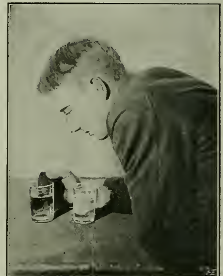
Fig. 20. This Shows Apparatus Arranged for the Accurate Testing of Cotton and Wool Content of Cloth, and One That is Used by Practically All Commercial Cloth Testers. One Glass Contains a Solution of Caustic Potash, or Caustic Soda, into Which is Immersed a Sample of the Wool to Be Tested. A Precipitate Indicates the Relative Amount of Cotton and Other Substances Present. Likewise When Cotton is Immersed in an Acid, a Precipitate Will Show the Relative Amount of Adulterants. See Also Fig. 7.
