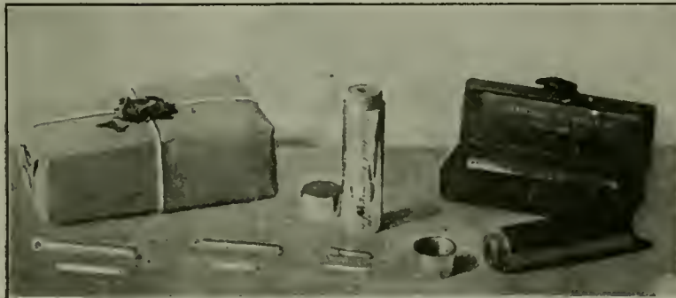
Method of Preparing Radium in Tubes For Use in Medical Work. The Three Small White Tubes Contain Radium Sulfate and Have Respectively 2,550 and 100 Milligrams of Radium Element Content. Beside them Are the Silver and Platinum Screens Used, Back of Which Is the Brass Carrying Tube, Together with a Package Ready for Shipment.
