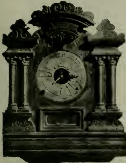
The Clock Fitted with Automatic Electric Bell-Ringing Switch. This Arrangement Has Given Entire Satisfaction in a High School for Some time, and Provides 18 Rings Between 9 A. M. and 4 P. M.
