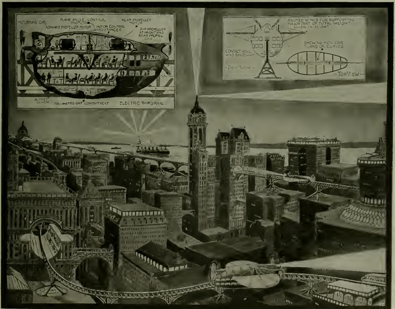
The Aerial Monoflier of Tomorrow—Equipt with Wings, Like an Airplane, It Will Skim Along Thru the Air, Guided by the Monorail. The Cars Are Propelled by Motor-Driven Propellers, Which Derive Their Power from Third Rails, as the Car Glides Along at Speeds of 200 to 300 Miles Per Hour. When In Motion the Entire Weight Is Practically Carried by the Wings, the Same as in an Airplane.
