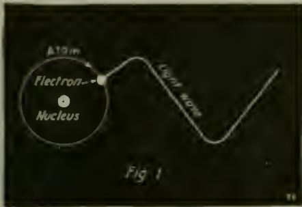
Diagram Illustrating the Old Theory of Light Produced by Electricity. In This Explanation the Electron is Considered as Continuously Producing Light Waves by Its Rotation. The Newer Theory of Light and Heat Waves is Shown at Fig. 2.
